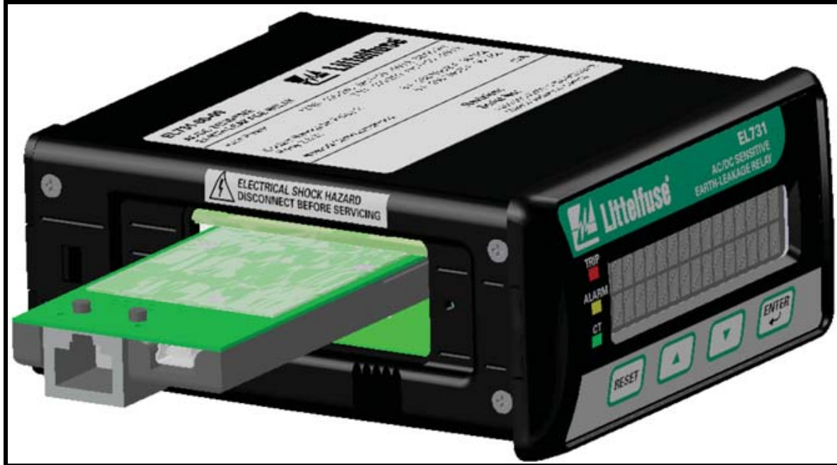
FIGURE 3 Firmware Upgrade Module (AC700-CUA-00) in an EL731.
